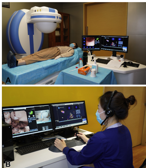
Figure 1. Noncontact magnetically controlled capsule endoscopy system. The system consists of a robotic magnetic arm (A), a workstation (A, currently bypassed), a capsule endoscope, a remote-control workstation (B), and an audiovisual exchange system (A, B).
